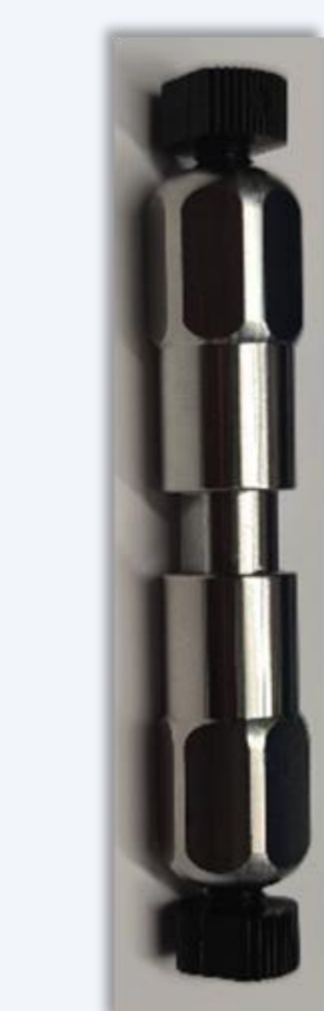
Figure 4. UHPLC column used as PBR (ID: 0.3 cm, length: 3 cm).
